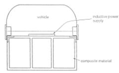
Figure 5.1. Cross-section of beam and vehicle
