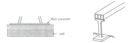
Figure 5.3. Ground foundation with slab
