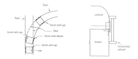
Figure 5.4. Switching with lever arm
