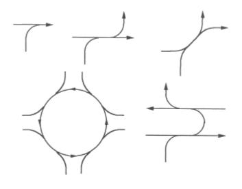
Figure 6.9. Types of single-level intersections
